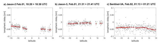
Fig. 1. Selected tracks of altimetry-derived  $K_{tr}$ -band ionospheric delay determination (black) and its smoothing by moving average with 80 s window (red).
